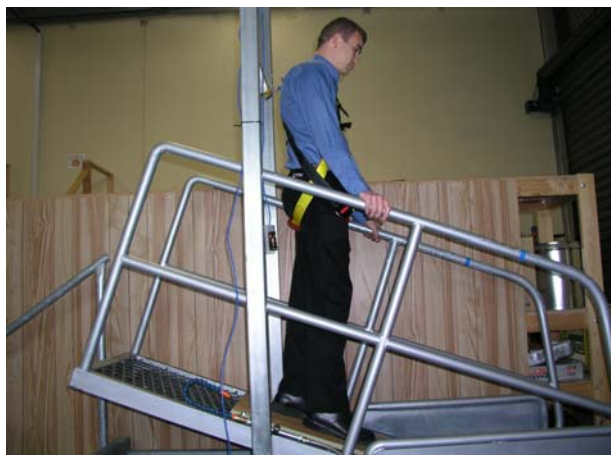
(b) Inclining ramp testing apparatus
